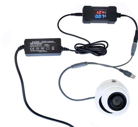
Fig 1 Shows camera current and voltage in normal mode
