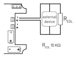
The  $10 K\Omega$  R EOL resistor monitors whether the cable has been damaged or the connection is no longer available.
